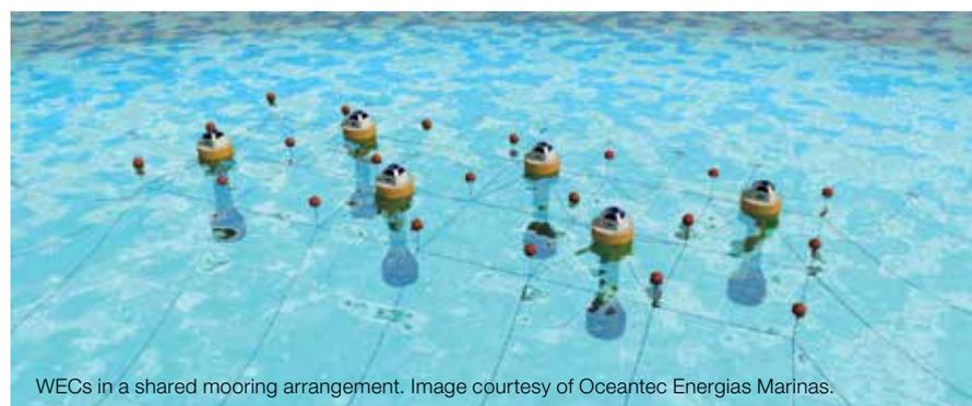
WECs in a shared mooring arrangement. Image courtesy of Oceantec Energias Marinas.
