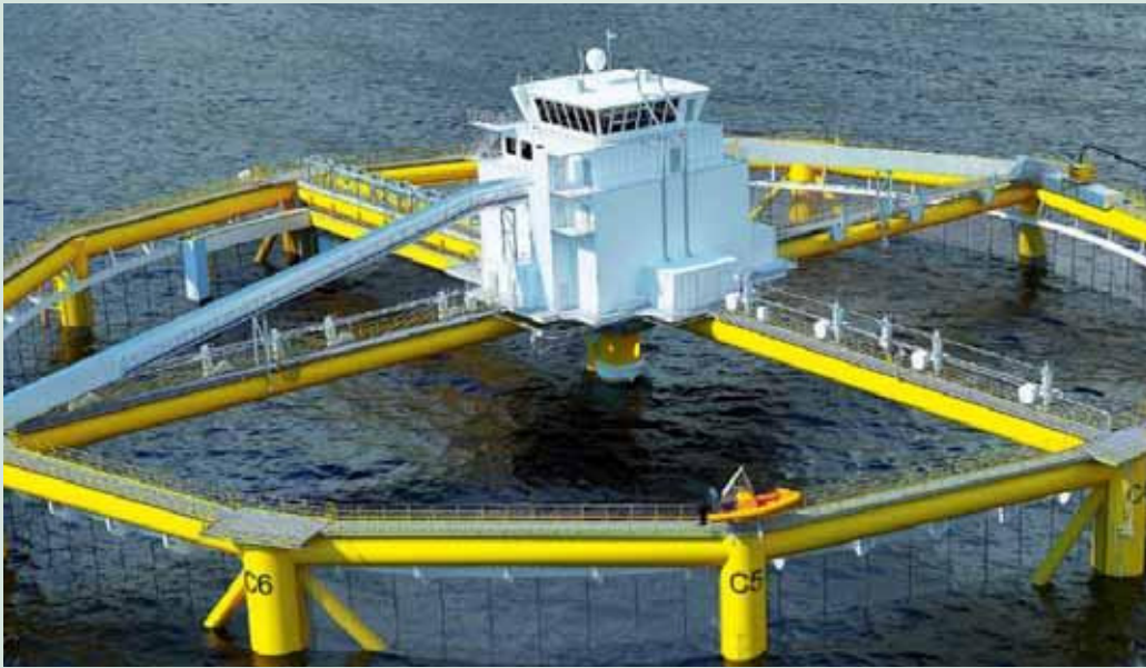
The expertise and technologies used in semi-submersible vessels in the offshore oil and gas sector can also be deployed in the development of fish farms.
